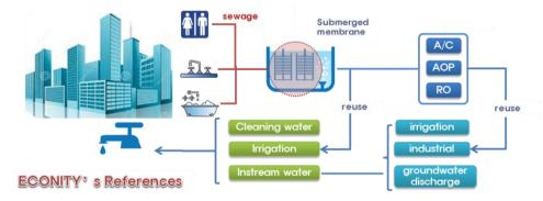
**Research Fields** 1 Membrane product—Design-Construction-O&M 2 Total water solution **Keywords** Membrane filtration, Waste Water treatment, MBR, Water reuse, Package system
